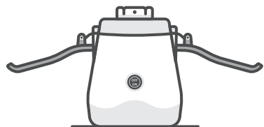
400-watt motor base with locking arms
